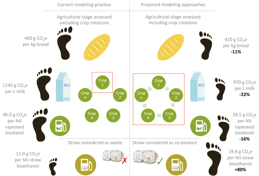
Figure 9 Comparison of product carbon footprints (PCFs) for wheat bread, cow milk, rapeseed biodiesel, and straw bioethanol using current modeling approaches: 1-year systems vs. crop rotation and straw as waste vs. straw as a co-product.
